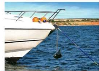
2 When the mooring line is through the bow roller, immersing the anchor prevents it swinging into the hull.
