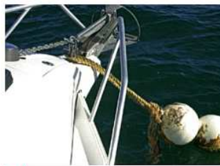
1 For extended mooring, the mooring line should run through the bow roller to prevent chafe.
